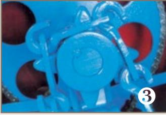
**Patz Drive Sprocket protects the chain, keeps the chain on and lasts for years.**
