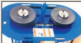
The tapered-bore drive pulley mounts to a 1-1/8-inch (29 mm) drive shaft with a greaseable flange bearing at the top of the drive tube. A lip seal below this bearing keeps contaminants out of the drive tube. The drive tube is filled with oil to lubricate the support bearings inside the tube and the bottom bearing.
